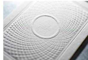
Fig. 8 Embossed paper tactile printing
